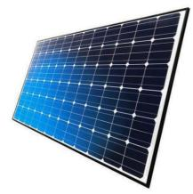
A monocrystalline solar panel is a solar panel comprising monocrystalline solar cells. These cells are made from a cylindrical silicon ingot grown from a single crystal of silicon of high purity in the same way as a semiconductor. The cylindrical ingot is sliced into wafers forming cells
